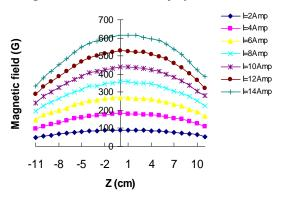
Figure (2): The experimental magnetic field profile as a function of coil current.
