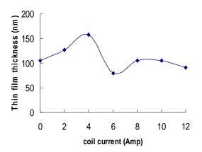
Figure (5): Thin film thickness versus current of Coil at constant pressure of  $7x10^5$  mbar.
