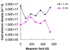
Figure (11): the influence of the magnetic field strengths on the cold electron density at different radial position from the cathode.
