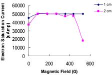
Figure (9): The influence of the magnetic field on the electron saturation current at different radial positions.
