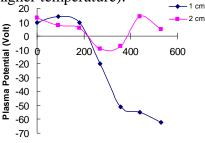
Magnetic Field (G) Figure (10): The variation of the plasma potential with increasing of magnetic field strengths for different radial position from the cathode.
