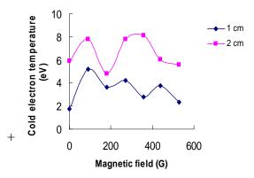
Figure (8): the variation of cold electron temperature with magnetic field strength at different radial positions.
