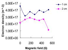
Figure (14): the influence of the magnetic field strengths on the electron density at different radial position from the cathode.
