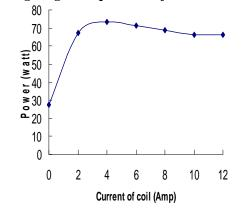
Figure (4): Curve of power of the system versus Current of coil at pressure of  $7x10^{-5}$  mbar.
