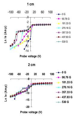
Figure (6): Ln I<sub>e</sub>-V curves at different radial Positions versus magnetic field strength.
