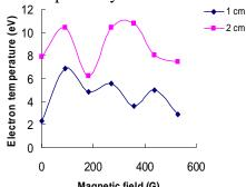
Magnetic field (G) Figure (13): the influence of the magnetic field strengths on the electron temperature at different radial positions from the cathode.
