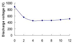
Figure (3): Behavior of discharge voltage versus coil current for abnormal glow discharge region at pressure of 7x10<sup>5</sup> mbar.
