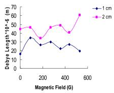
Figure (15): the influence of the magnetic fieldstrength on the Debye Length at different radial positions from the cathode.
