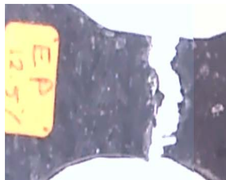
Figure (11) The fracture in EP-12.5%wt CCF
