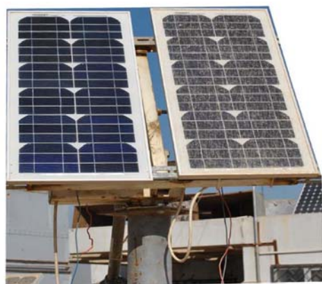
Fig.(1) Two solar panels(reference and dusty panel under test) with two-axis solar tracking system used in the experimental measurements.
