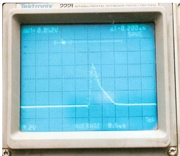
Fig. (4) Represents laser semiconductor pulse duration show by storage Tektronix oscilloscope where x-axis =0.5 usec/div, y-axis=0.2 V/div.
