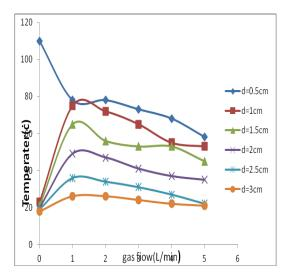
Fig(4): Dependence of the gas temperature on the gas flow rate at various distance
