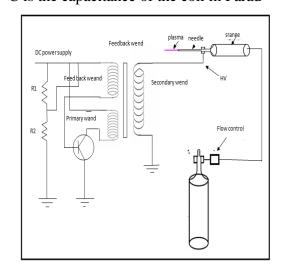
*Fig.(2): Schematic diagram of a non-thermal plasma source*
