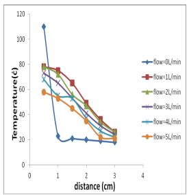
Fig (3): Dependence of the gas temperature on the axial distance between the thermometer and the tip of the needle for various gas flow rates
