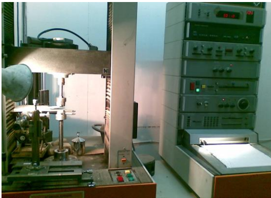
Fig.3: Instron testing machine with DCB test
