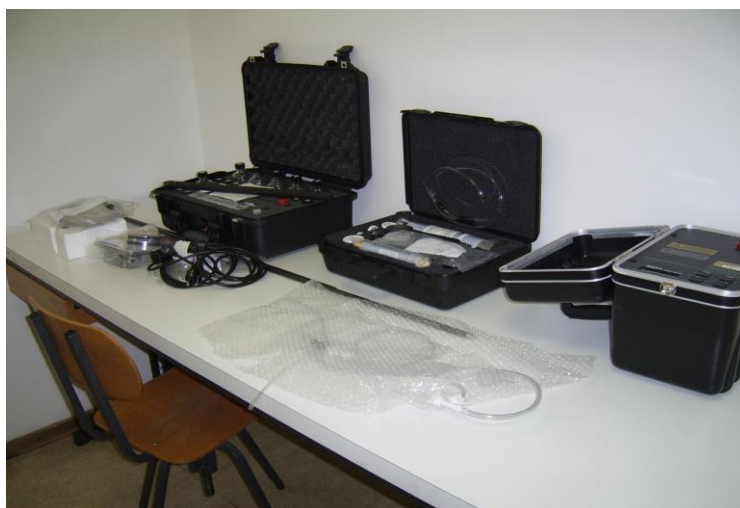
Fig.2: The RAD-7 soil-gas setup, including the electronic Radon monitor
