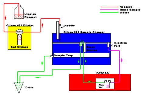
Fig. 1: Tubing diagram of the kinetic phosphorescence analyzer [10].
