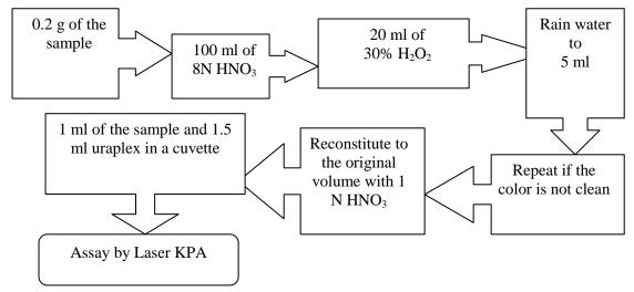
Fig. 2: Chart of radiochemical extraction of uranium [9].
