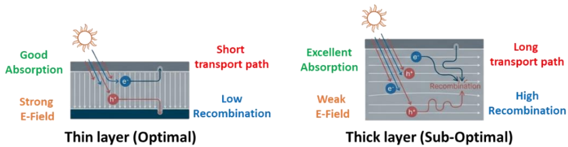
Figure 2: The differences between thin and thick active layers in different perspectives.
