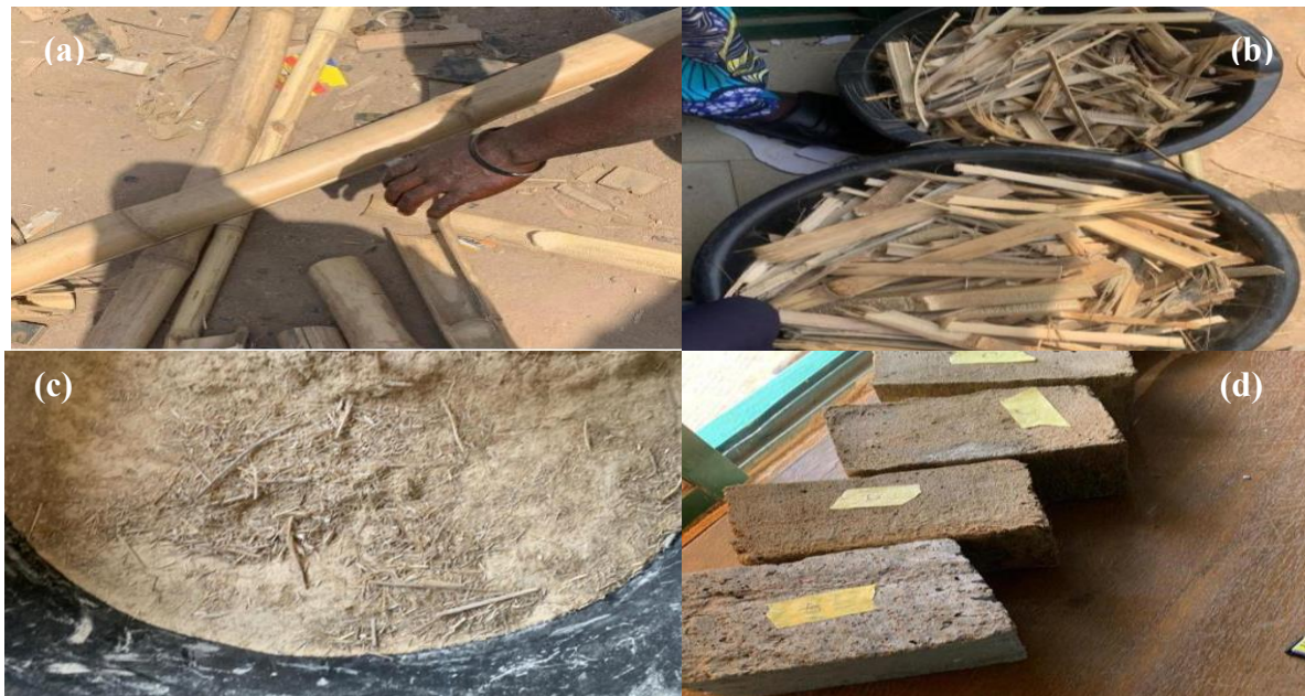
Figure 1: (a) Bamboo sticks before cutting into smaller pieces, (b) Bamboo pieces after treatment with NaOH, (c) Pulverised Bamboo, and (d) Mortar Samples.
