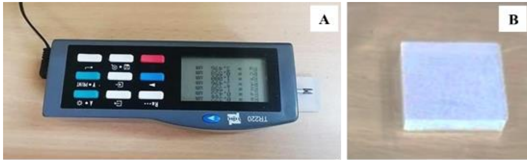
Figure 4: Surface roughness test (A) Contact profilometer, (B) Surface roughness test specimen.
