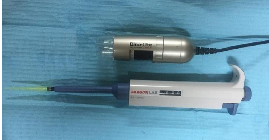
Figure 2: The Dino-Lite digital microscope and the micropipette used in the wettability test.
