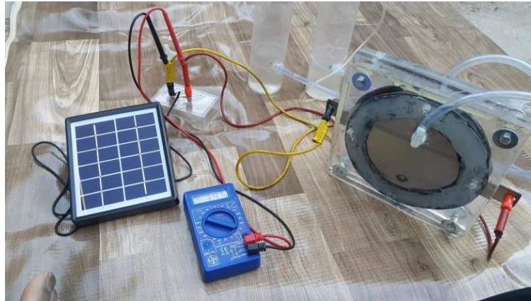
Figure 2: The final construction part of dry HHO cell.
