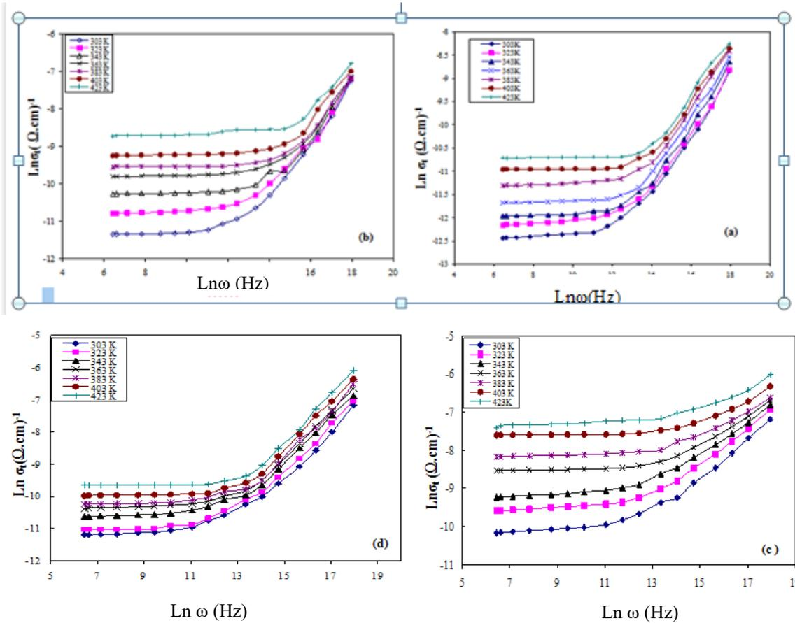
Figure 4:  $\ln \sigma_i$  as a function of  $\ln \omega$  for (a) pure PANI, (b) 0.5 M, (c) 1M, and (d) 2M  $\text{H}_2\text{SO}_4$  at different temperatures.
