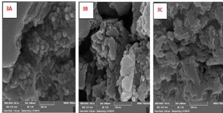
**Figure 3: SEM images of the prepared PANI in (A) water, (B) 1M  $H_2SO_4$ , and (C) 2 M  $H_2SO_4$ .**
