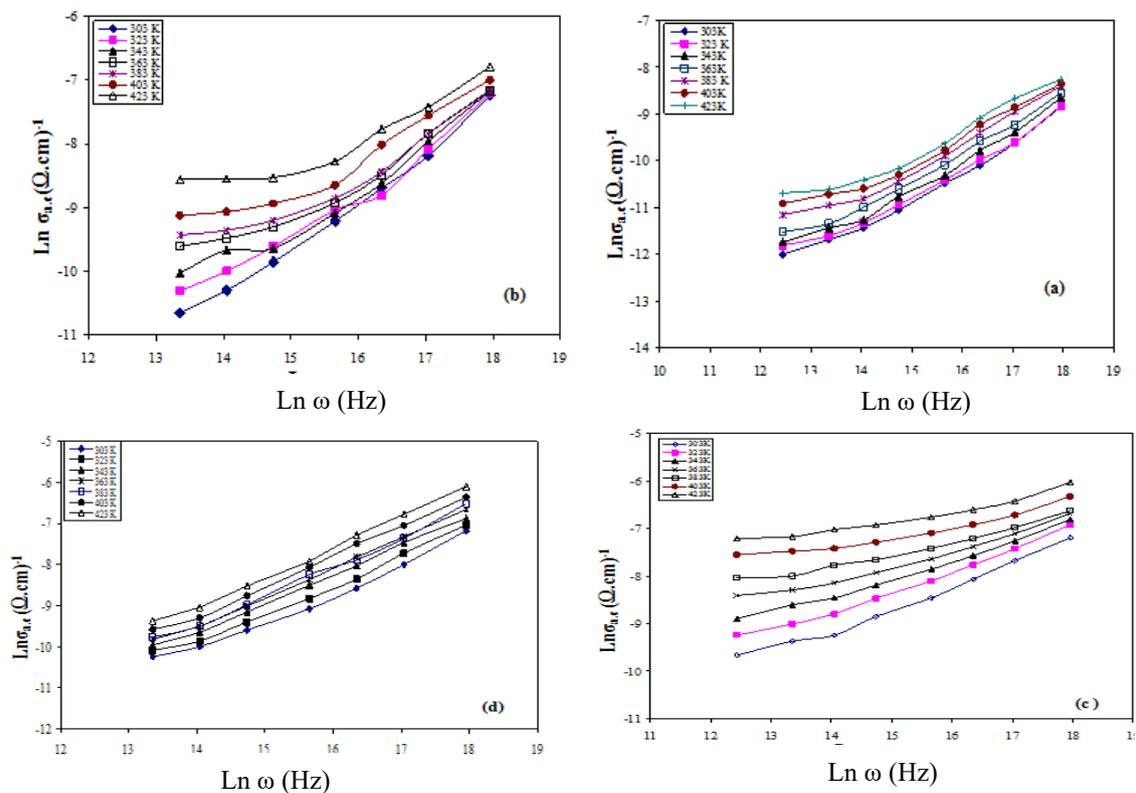
Figure 5:  $\ln \sigma_{a.c}$  as a function of  $\ln \omega$  for (a) pure PANI, (b) 0.5 M, (c) 1M, and (d) 2M  $\text{H}_2\text{SO}_4$  doping at different temperatures
