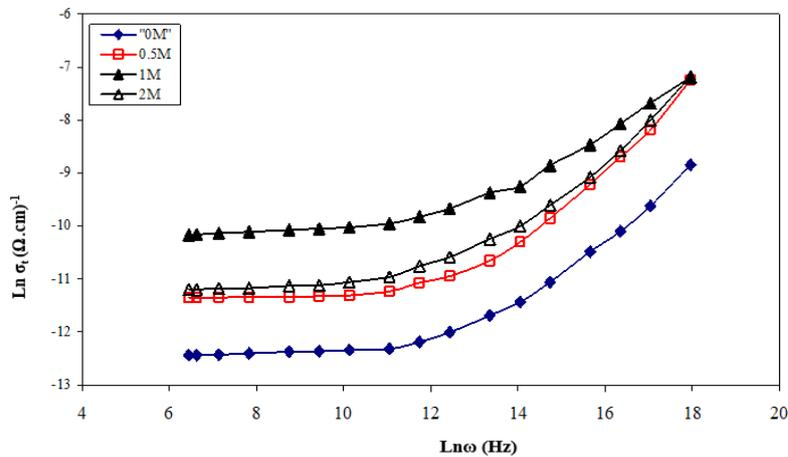
**Figure: 8 Frequency dependence of conductivity for different  $H_2SO_4$  molarity.**
