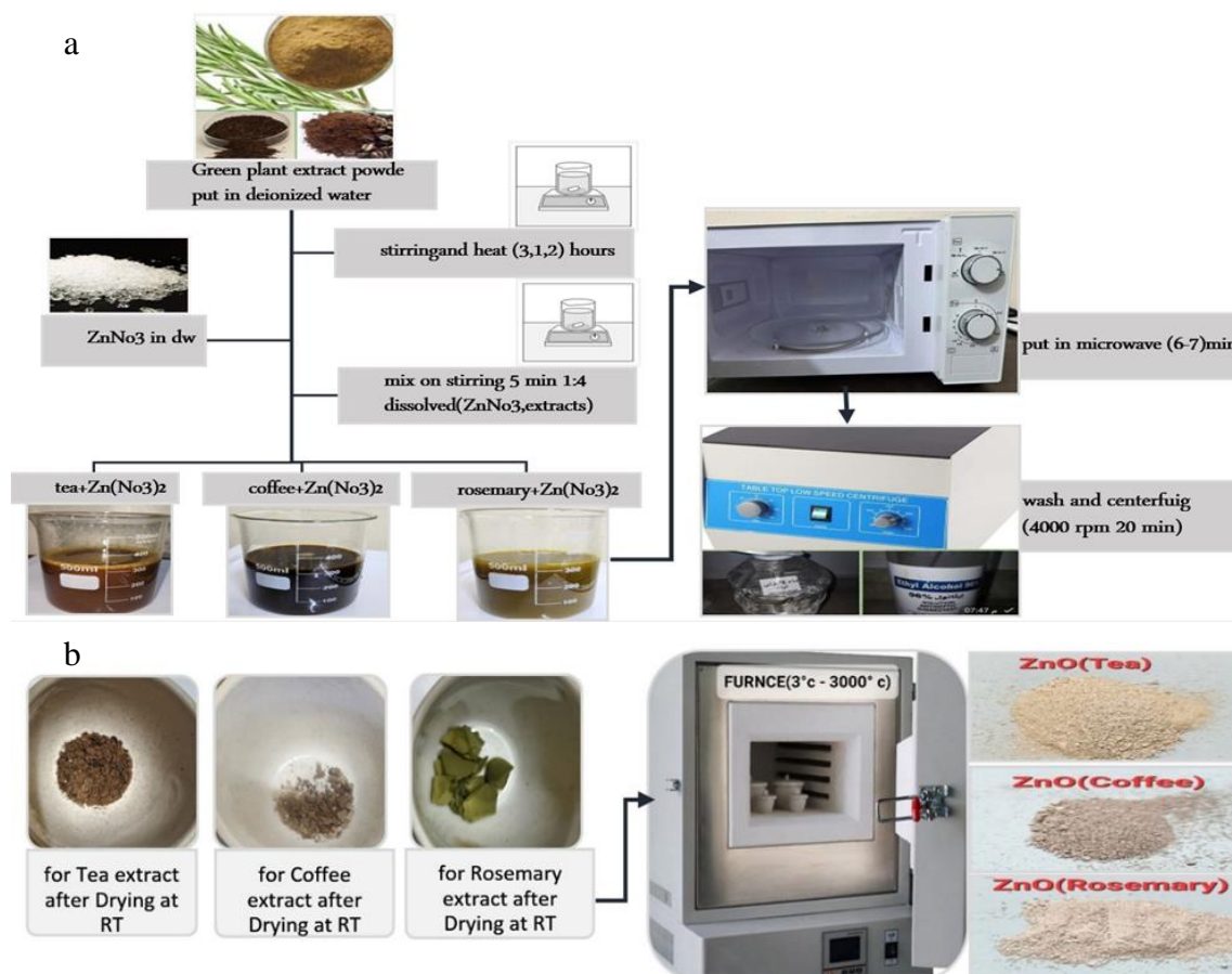
Figure 1: (a) Steps of preparing the plant extract and combine it with zinc nitrate to prepare zinc oxide NPs (b) Zinc oxide NPs powder synthesized by green synthesis.
