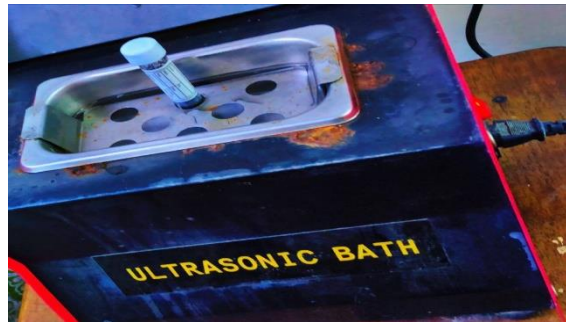
Figure 3: Mix grapheme with ethanol alcohol C_2H_5OH by using an ultrasonic bath device.
