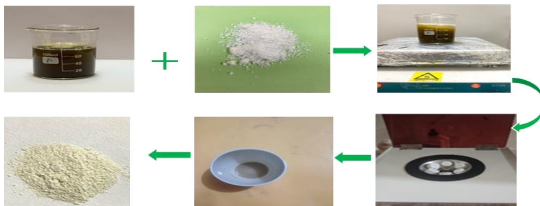
Figure 3: preparing pure ZnO NPs using Ficus carica (fig) leaves.
