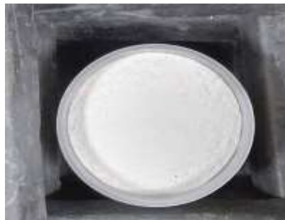
Figure 4: Flour sample in Marnelli Beaker inside the shield.
