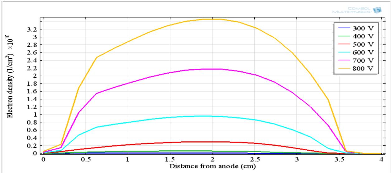
**Fig. 6: Spatial profiles of electron density as a function distance from anode at different discharge voltages.**
