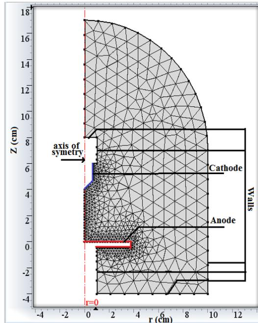
**Fig. 2: Definition of 2D axial-symmetric model boundaries identical with experimental chamber.**
