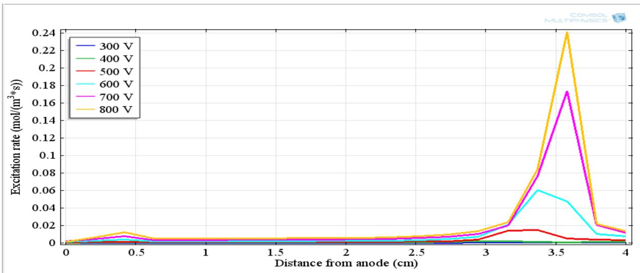
**Fig. 12: Excitation rate as a function distance from anode at different discharge voltages.**
