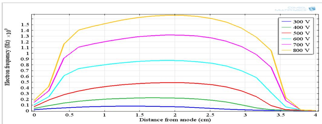
**Fig. 7: Electron frequency as a function distance from anode at different discharge voltages.**
