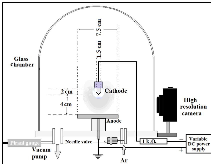
*Fig. 1: Schematic for experimental setup.*
