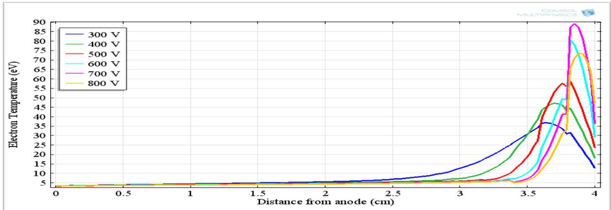
Fig. 8: Electron temperature as a function distance from anode at different discharge voltages.
