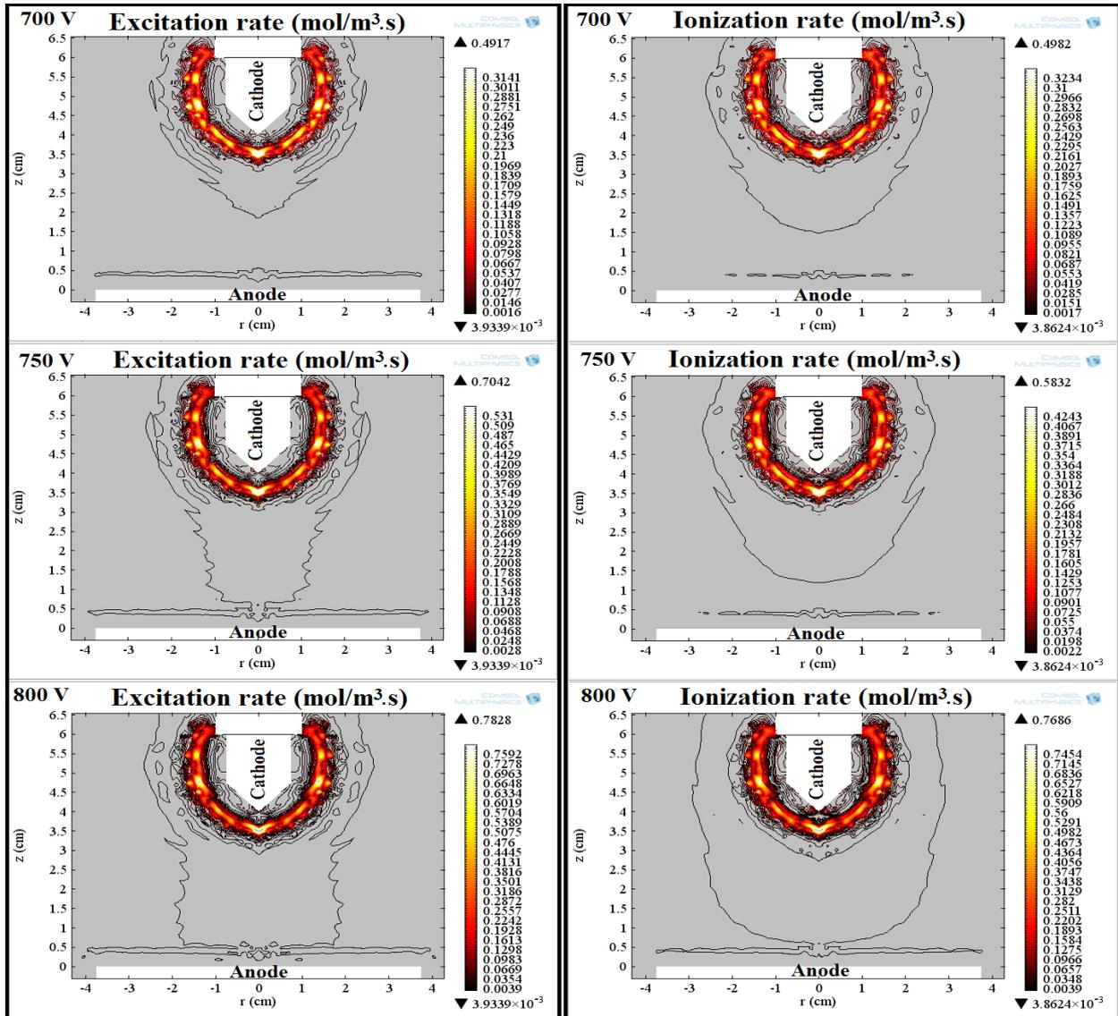
Fig.10: Distributions of excitation rate and ionization rate as a function applied voltage.
