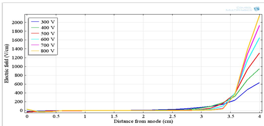
**Fig. 4: Electric field profile distribution along the axial distance from anode.**
