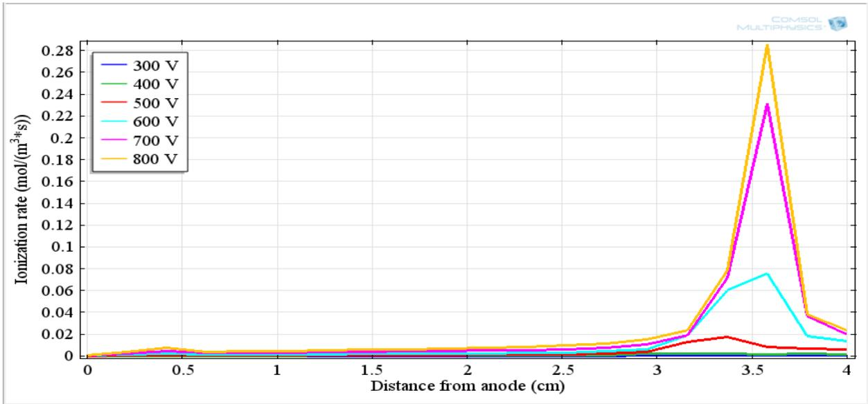
**Fig. 11: Ionization rate as a function distance from anode at different discharge voltages.**
