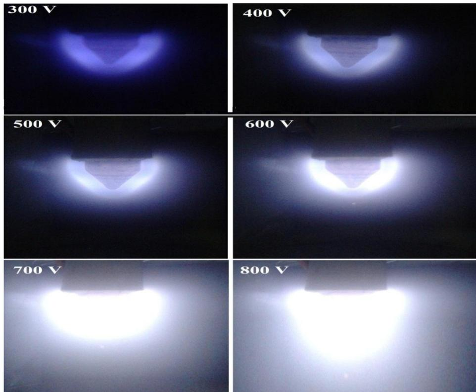
**Fig.13:** Image during formation of glow discharge as a function applied voltage.
