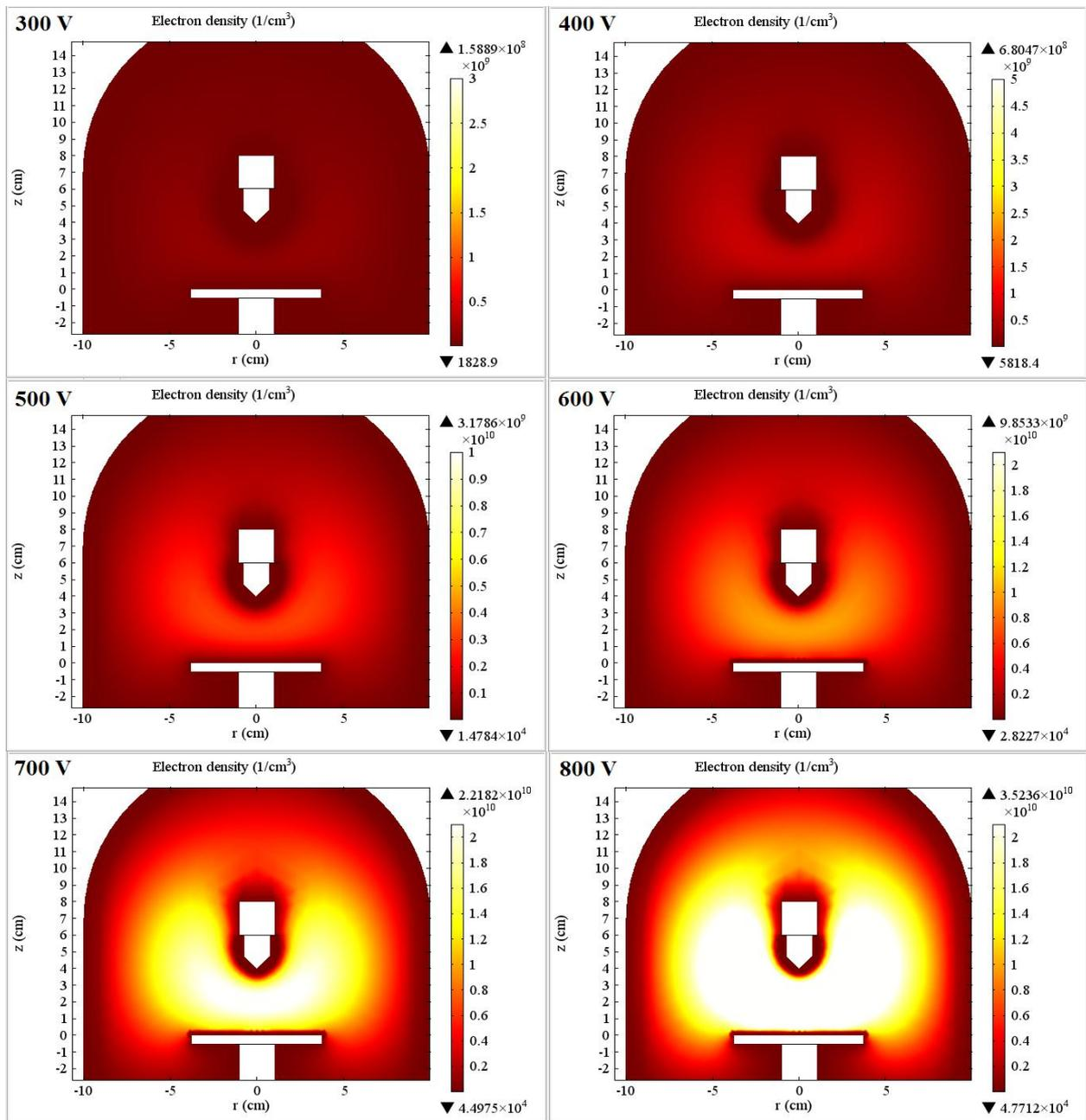
**Fig. 5: The distribution of electron density with different applied voltages.**
