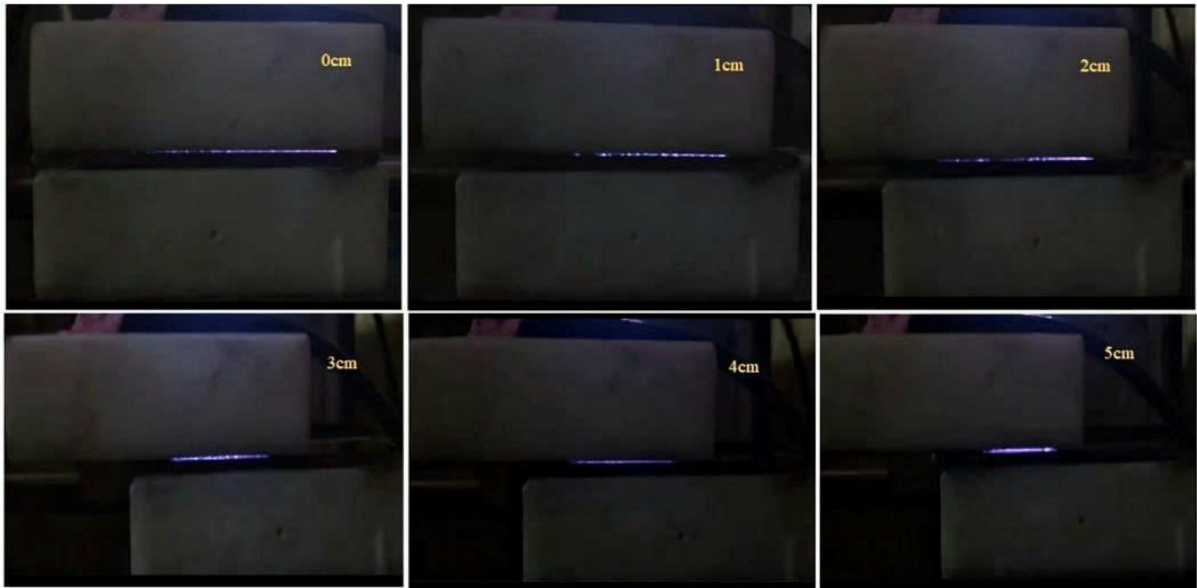
Figure 3: Influence of horizontal distance on the plasma formed in the DBD actuator with the magnetic mirror configuration.
