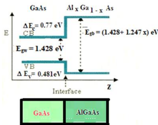
Figure 2: Band alignment of (GaAs/Al x Ga 1-x As) in the direct-gap range.
