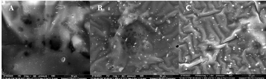
**Figure 4:** SEM images at 1300x (A) control samples, (B) soft liner with 2% CeO<sub>2</sub>, (C) soft liner with 3% CeO<sub>2</sub>.
